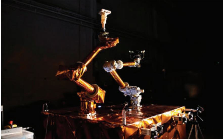
Flight-scale manipulator arms on the robotic operations test-bed (ROTB) for the RSGS robotic payload are on display during the preliminary design review in July 2018.
