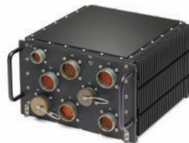
Northrop Grumman is building 42 6U VME-based conduction-cooled Gen III mission computers for the U.S. Marine Corps AH-1Z Viper combat helicopter.
